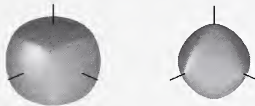
Figure 1. Equilibrium shapes for materials with cubic anisotropy. These shapes are energy minimizing surfaces that are the anisotropic versions of soap bubbles (the isotropic case).
